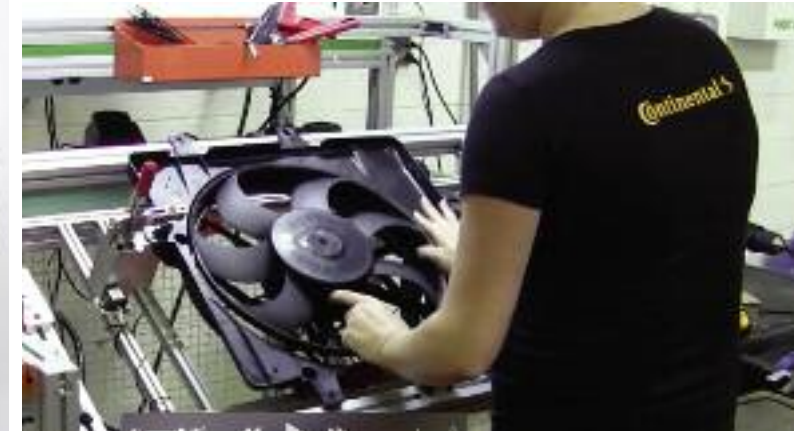
A Continental engine cooling fan is assembled and tested at the company's Allentown, Pa., facility.
